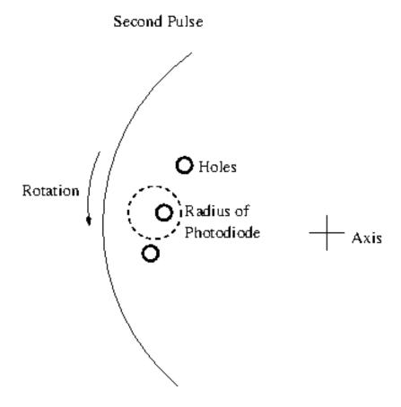
Please note that the difference in radius from the axis (center) of the disk is smaller than the aparture of the PhotoDiode. In reality, more than two holes can flash by and be 'seen' by the PhotoDiode. We use two to simplify what is happening.
