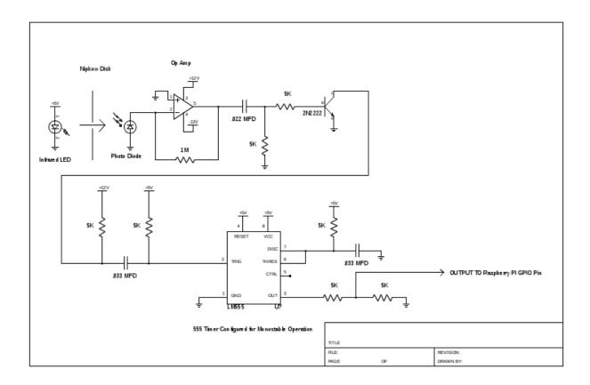
The LED and PhotoDiode are at the upper left hand corner of the schematic. The photodiode feeds an OP-Amp which provides current gain. The OP-Amp feeds a 2N2222 transistor that inverts the signal. The inversion is required because the LM555 timer requires a negative going pulse and the OP-Amp puts out a positive going pulse.
