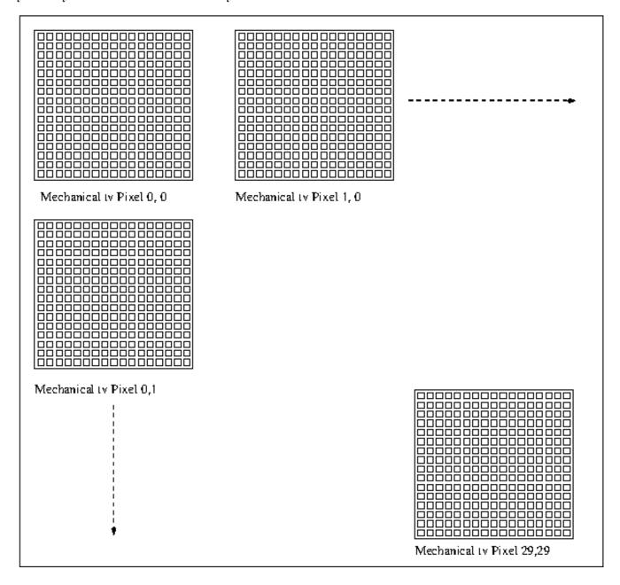
After each image is converted for size, the next step is cartesion axis conversion. In a GIF file, the images are arranged so that the pixels start at the upper left hand corner of the image and proceed horizontally from left to right for each line. The lines in turn count up from top of image to the bottom.
