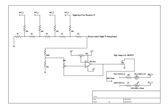
The resistor ladder is at the upper left hand corner of the schematic. There was no real logic in selecting the resistor values for the ladder. I merely found a bunch of resistors at the Spark Museum's workshop and used them. The only criteria was that the resistors from each of the bit signals are supposed to be twice the value for those in the series string from ground to the output.
