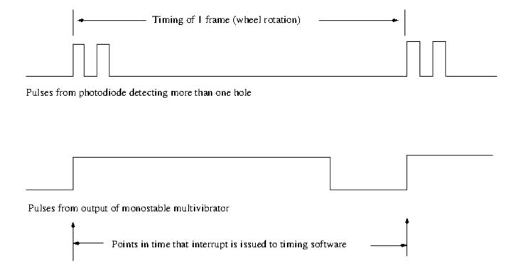
The duration of the monostable multivibrator is set to be long enough to cover the timing of about 7 holes. We estimate that about four holes are 'seen' due to the size of the aparture of the PhotoDiode.
