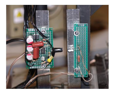
This is the optical sensor assembly for generating the timing signals from the kit mechanical television. The Nipkow disk is between the two printed circuit boards; it is difficult to see because it is viewed from its edge.
