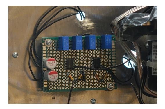
There are four potentiometers on the signal processor board. In order starting from the left (where the two electrolytic capacitors are:
