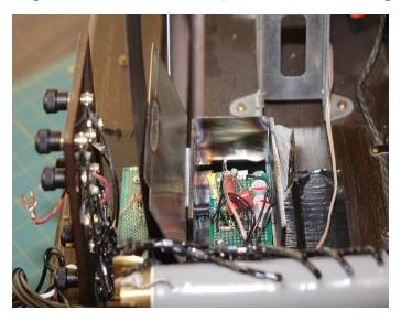
Here is the optical sensor circuit board with the shield open.
