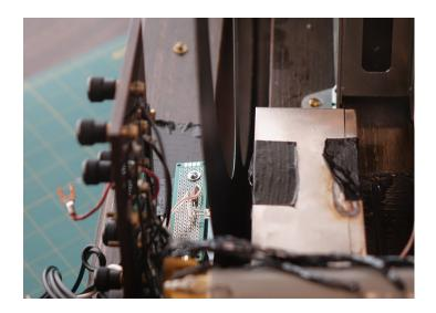
Due to excessive electrical noise from the motor of the Baird, the optical sensor circuit board has to be shielded. In the above photo, the infrared LED assembly is to the left and the metal shield with the duct tape is to the right. The Nipkow disk is in the center (hard to see due to being viewed from the edge).
