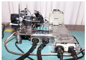
The two multi pin octal electrical sockets in the center are for the timing and video signals; the one on the left is for the kit mechanical television and the one on the right is for the Baird Televisor. T
