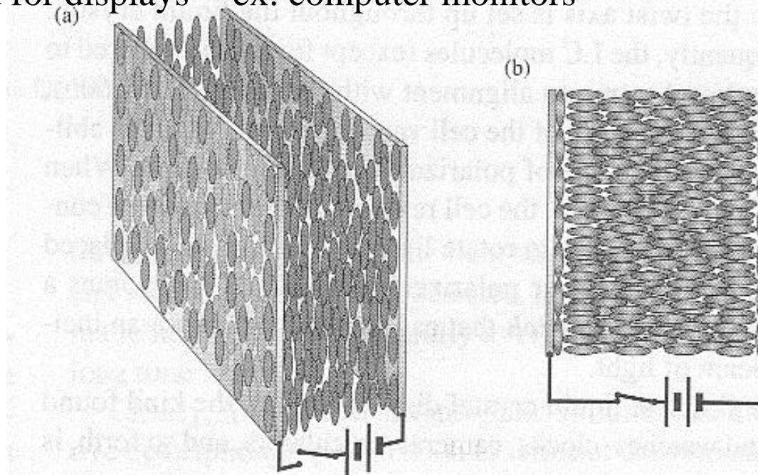
**Figure 8.59** (a) A nematic liquid crystal between two transparent electrodes. The long molecules align parallel to a set of microgrooves on the inside faces of the two electrodes. (b) When a voltage is applied, the molecules rotate into alignment with the field.
