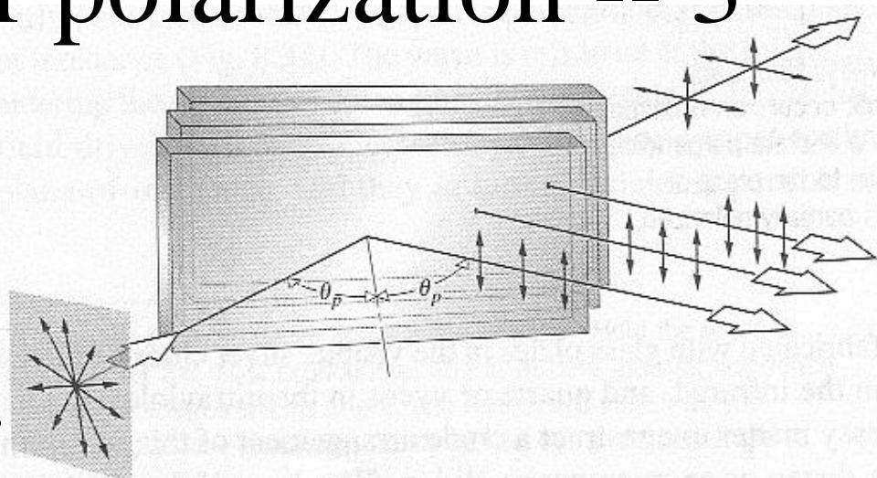
Figure 8.33 The pile-of-plates polarizer.
