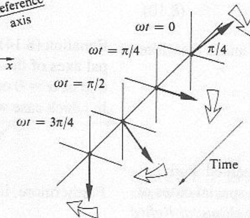
**Figure 8.3** Right-circular light. (a) Here the electric field, which has a constant amplitude, rotates clockwise with the same frequency with which it oscillates. (b) Two perpendicular antennas radiating with a 90° phase difference produce circularly polarized electromagnetic waves.
