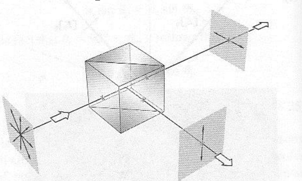
**Figure 8.34** A polarizing cube contains a multilayer dielectric thin film structure on its diagonal face. Reflection from that structure polarizes the incident light, much as would a pile-of-plates.
